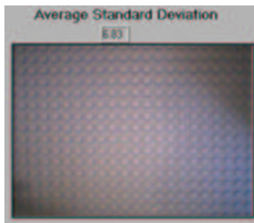
Figure 5.10: Average standard deviation of a piece of gray LEGO plate
