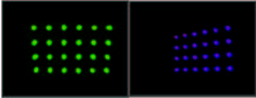
Figure 3.5: Calibration plate as seen by the center and side cameras
