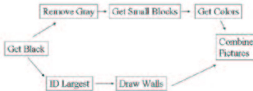
Figure 5.6: Flow chart of the block recognition process
