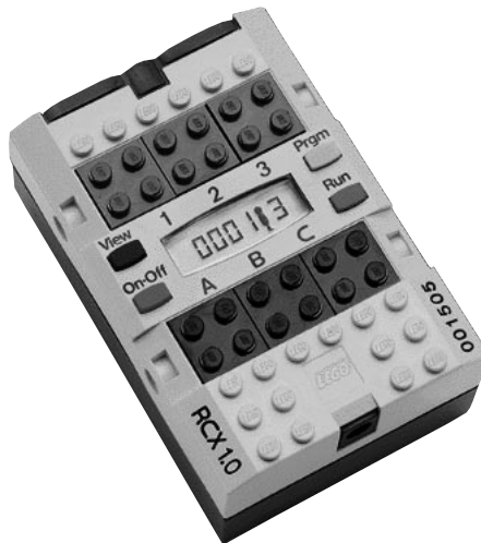
Figure 1. The RCX can store up to five different programs. Ports 1, 2, and 3 take input from sensors, while Ports A, B, and C supply power to motors or lights. (The RCX is approximately 2.5 inches by 3.75 inches.)
